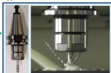
Chips are ejected smoothly if the outside diameter of the holder is reduced.
