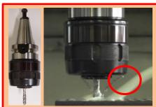
Chips hit against the holder and are not ejected smoothly if the outside diameter of the holder is too large.
