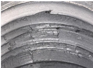
Torn internal threads surface after being tapped by a SP-PT 1/4 tap.
