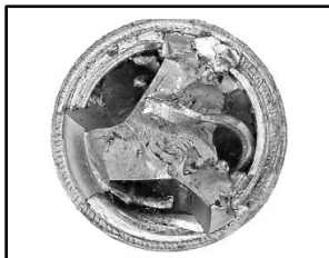
Condition of tap breakage
