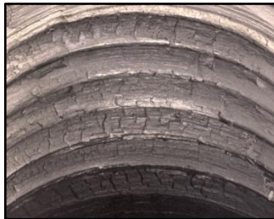
Surface of internal threads after threading
