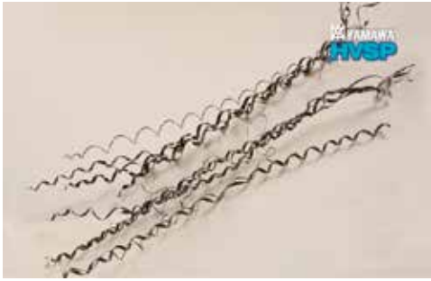
Ejected chips by large size taps
